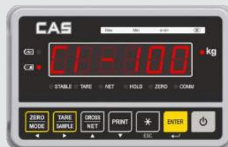
LED display (Character Height: 25mm, 6 digits)
